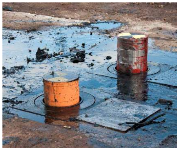
Bollards Operational After Impact
